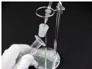
Figure 37. Installing the outlet dripper to the dripper stand.
