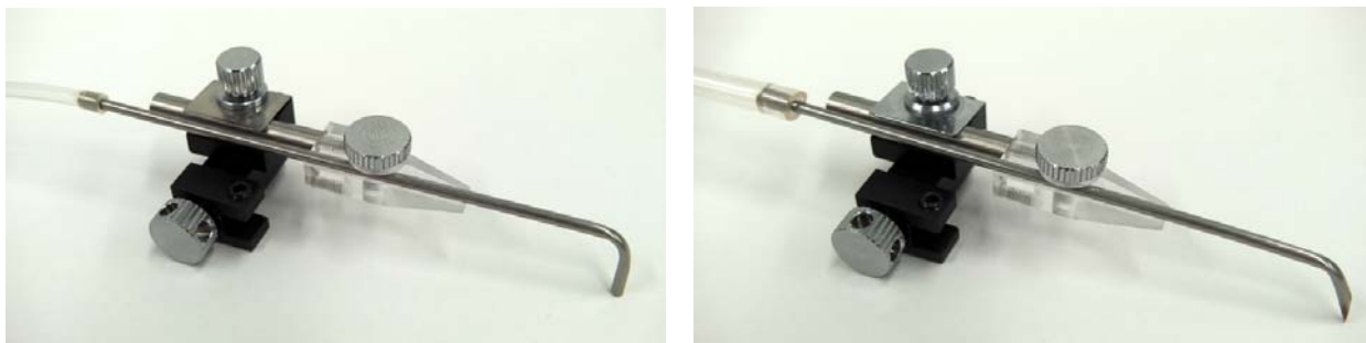
Figure 11. Inlet (left) and Outlet (right) Pipes installed to the Perfusion Pipe Holders.
