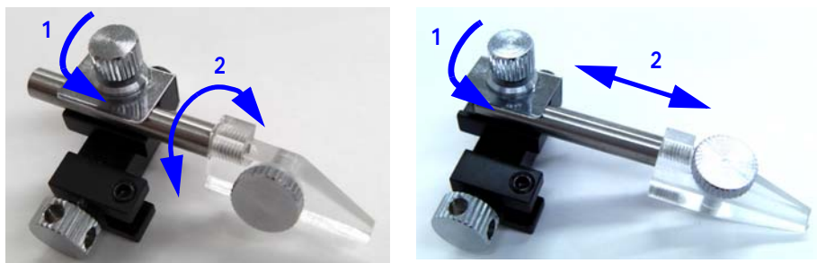
Figure 3. Functions for the Top screw. Loosening the screw and rotating the bar will change a height for the pipe/ Ref. Electrode (left). Loosing the screw and sliding the bar will change the distance of the pipe/ Ref. Electrode to the MED Probe chamber (right).
